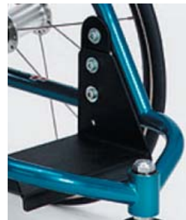
Figure 3. Screw for the footrest.
